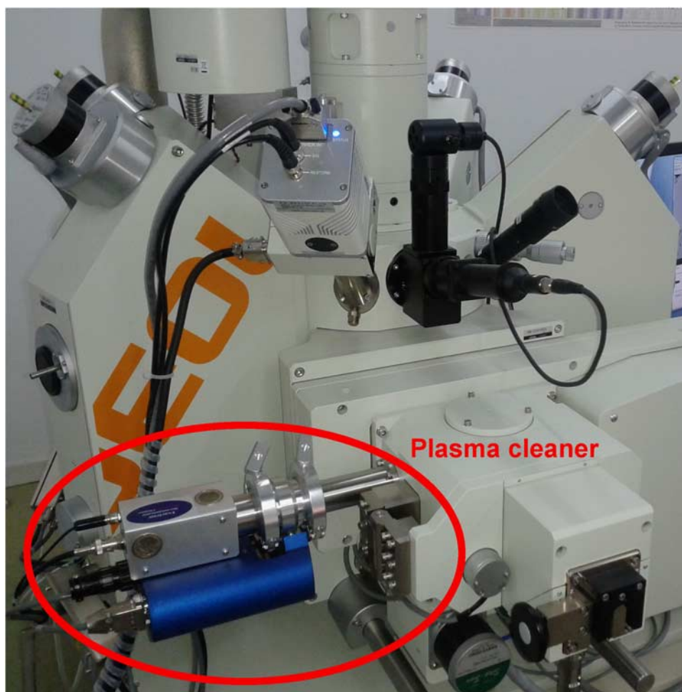
Figure 9. Modern electron microprobe instrument (JEOL JXA-8230)* equipped with a radio-frequency plasma cleaner mounted in the prechamber.
