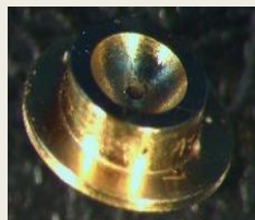
Specimen carriers - Gold plated copper - Dome-shaped indentation
