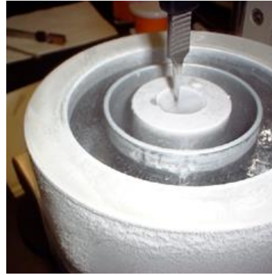
Cryo fixation of the hydrated sample By plunge freezing
