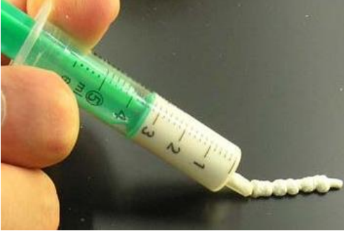
Preparation of a CPC/gelatin sample used as injectable bone substitute
