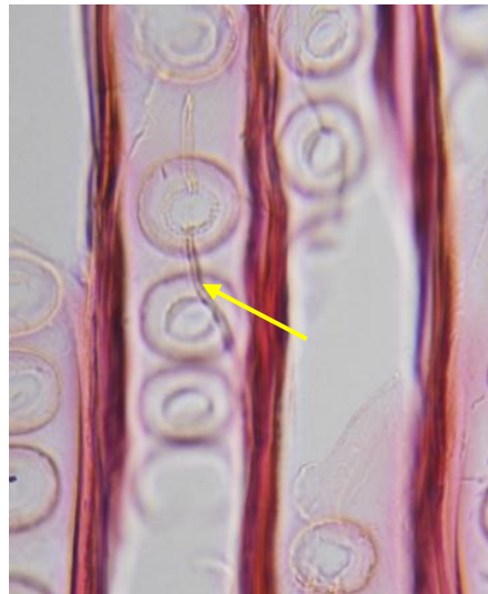
Light microscopy and SEM images of hyphae in wood
