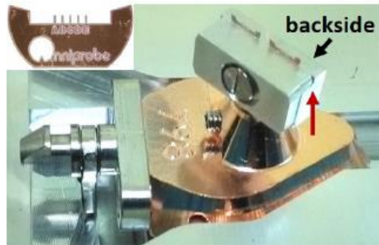
Figure 1: Modified SEM-TEM grid holder for FIB preparation of samples on TEM grids (Cu TEM-5-post half grids, top left), TKD and APT analysis. The backside is diminished to be suitable for TKD analysis. The step facilitates transfer and alignment of the grids. The stub is thinned to fit in the conventional APT holder.
