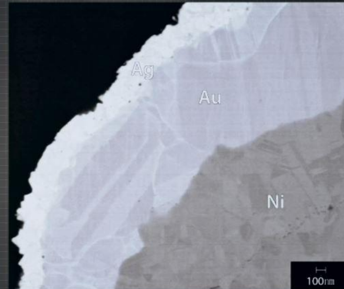
BSE Image at ×30K Specimen: Powder
