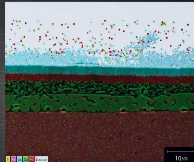
EDS Image at \times 2K Specimen: Layered structures (MLCC)
