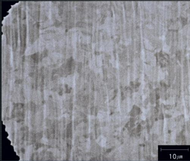
BSE Image at \times 1.5K Specimen: Cu Alloy
