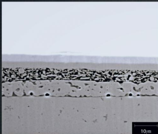
BSE Image at \times 2K Specimen: Layered structures (MLCC)
