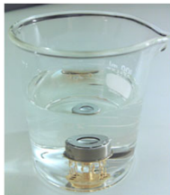
Si 3 N 4 Window, Impervious to water
