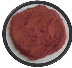
Copper (Cu) \alpha = 16.7 \times 10^{-6}/\text{K} k = 400 \text{ W/m.K}
