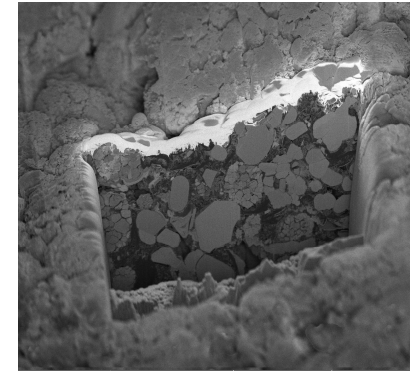
Ga + FIB: 50 \mu\text{m} wide cross-section of a Li-ion battery electrode
