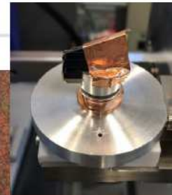
CIGS- solar cell sample preparation for SEM cross section analysis
