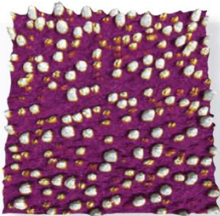
AFM conductivity image of GaAs quantum dots, 700 nm scan. Courtesy of T. Jones, U. Warwick.
