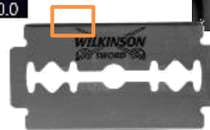
Razor blade edge imaged at 2 Hz (100 \mu\text{m} scan in 130 seconds)
