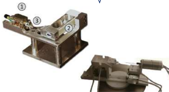
HELIOS 660 + EDS, EBSD + Platines Traction < 20N
