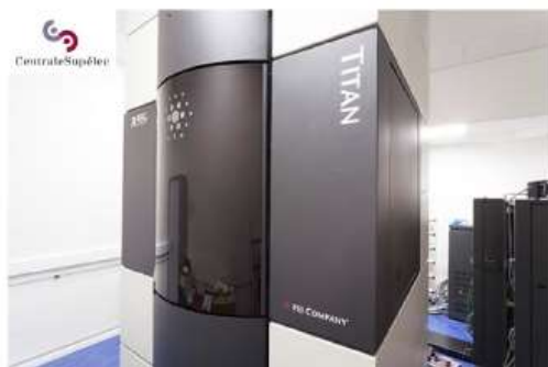
TITAN3 G2 + EDX, EELS + Platine Traction GATAN
