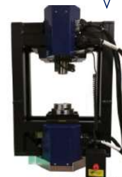
Tomographe RX NSI + Platine Traction/Torsion
