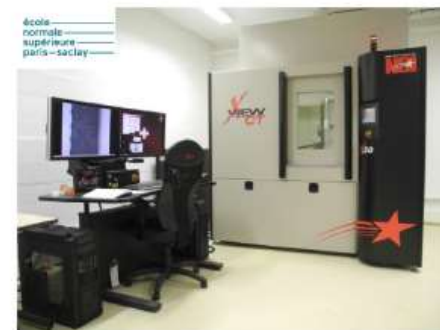
Tomographe RX NSI + Platine Traction/Torsion
