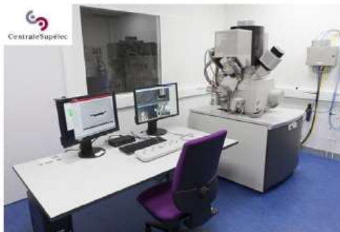
HELIOS 660 + EDS, EBSD + Platines Traction < 20N
