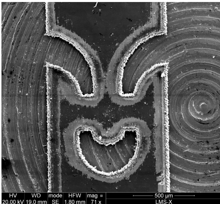
Heat affected zone
