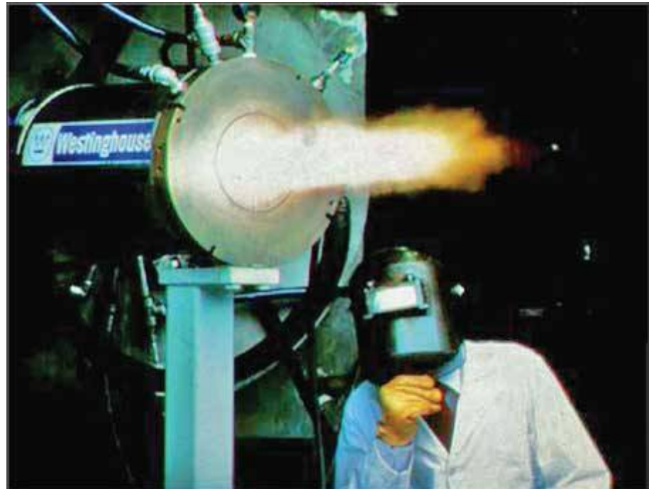
Westinghouse Plasma Corporation plasma torches that burn at over 12,000° F are used in plasma gas
