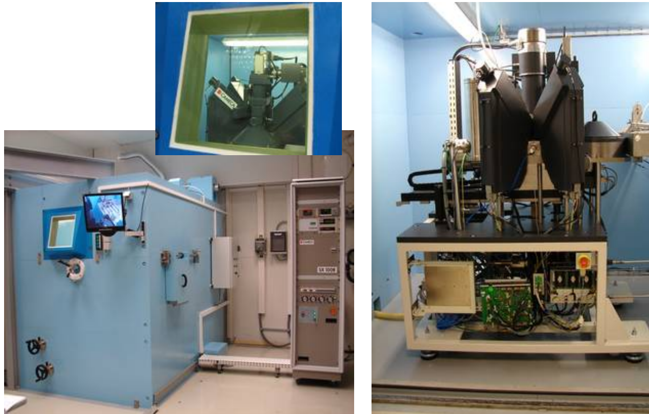
Views of the Cameca SX100R electron microprobe for the analysis of irradiated nuclear fuel at the Institute for Transuranium Elements.
