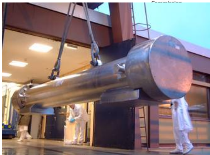
Irradiated fuel rods are transported in shielded containers
