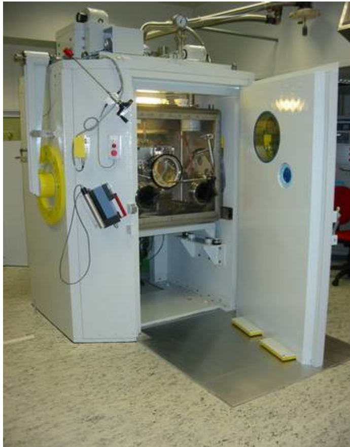
Front view of the installation showing the lead cell and glove box.
