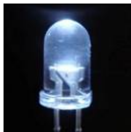
White LEDs (with yellow phosphors)
