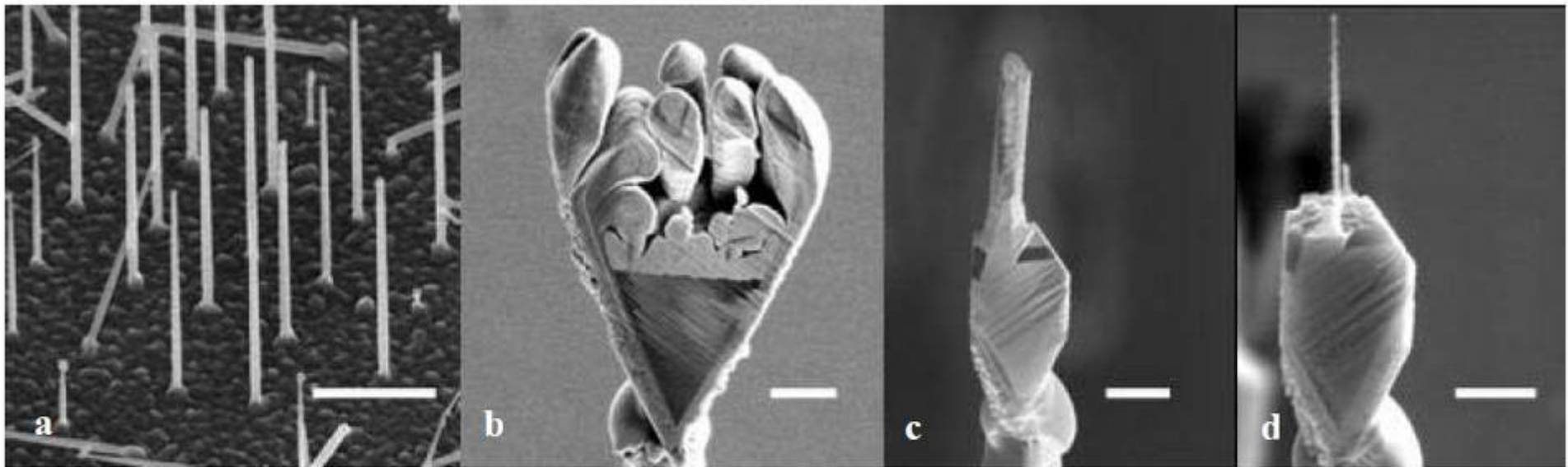
FIG. 1. (a) As-grown NW array. (b) Extracted wedge of Ni protected NWs attached to a microtip post. (c) Same wedge after FIB milling to isolate single NW for analysis. (d) NW after Ni removal via sulfuric acid etch. Note: All scale bars 2\mu in length.
