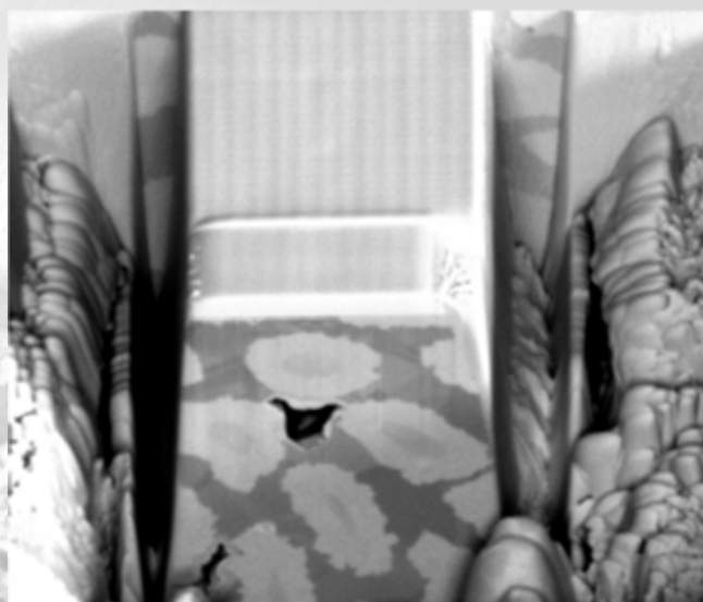
Automated milling and imaging of 170 slices (10h)
