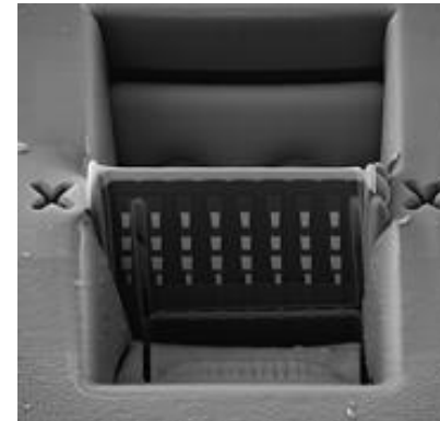
Sample preparation (here thin sample for S/TEM)
