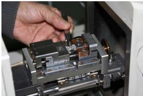
Fig. 3. Loading device with a sample to be furnished inside the SEM.
