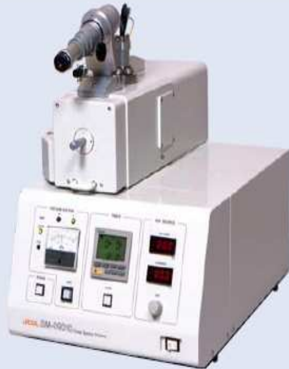
Fig. 2 Cross section polisher (CP) SM-09010
